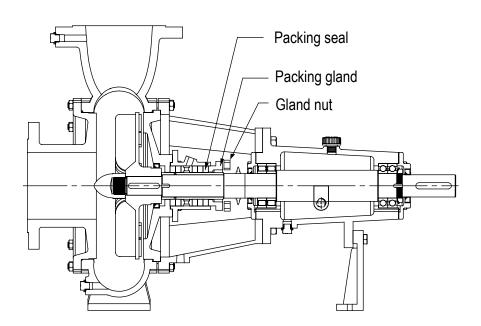
The location of the packing seal, the stuffing box and the packing gland on the pump. The design of the shaft seal housing .,/does, however, depend on the individual pump application.
