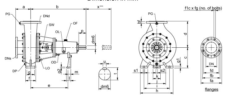
X\*\*\* distanace necessary for dismantling of bearing bracket with impeller
